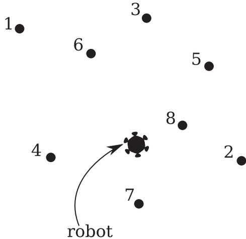
**Fig. 1.** The landmark order detector gives the cyclic order of the landmarks around the robot. Note that only the cyclic order is preserved, and that the sensed angular position of each landmark may be quite different from the real one. Thus, the robot knows only that the sequence of landmarks detected is  $[7,2,8,5,3,6,1,4]$ , up to a cyclic permutation.
