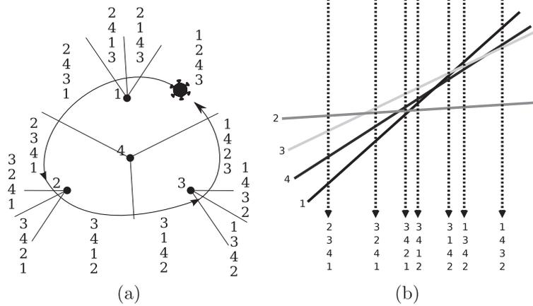
**Fig. 5.** Retrieving the permutations that encode the configuration of landmarks. In (a) the robot travels outside the convex hull of a set of landmarks. This is naturally expressed in the dual line arrangement in (b).
