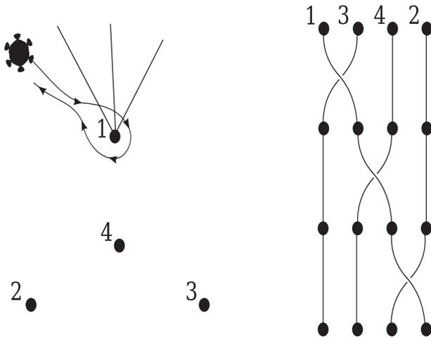
**Fig. 10.** Encoding the sensor history with braids. There is a natural description of the information space of  $n$  landmarks with the braid group on  $n$  strands,  $B_n$ . Each strand represents a landmark, and each crossing represents a change in the circular order. In the figure, the robot follows a path that surrounds landmark 1. The changes in the circular order are encoded with the braids on the right.
