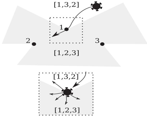
**Fig. 4.** Triangle orientation error. A small control error may find the wrong orientation for the triangle. On the bottom, if the robot follows the top-left arrow, the orientation is not computed correctly.
