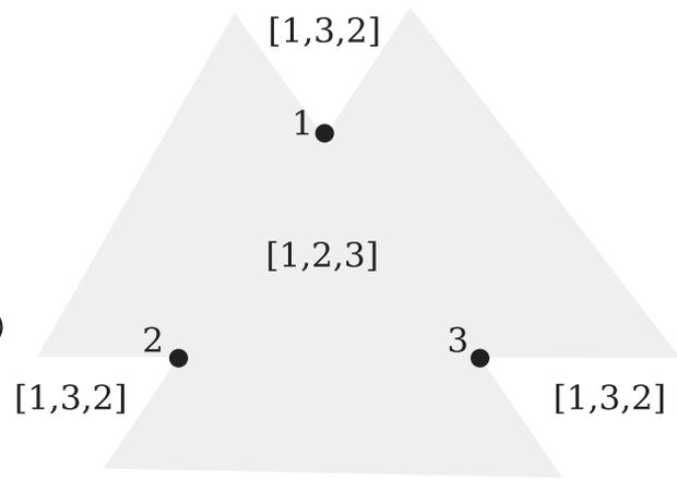
**Fig. 3.** Cyclic permutations of three landmarks. Purely by sensing, the robot cannot even know if it is inside the convex hull defined by the three landmarks. Nevertheless, the orientation of the triangle (the counterclockwise cyclic order of the landmarks as sensed from inside their convex hull) can be determined with an information state.
