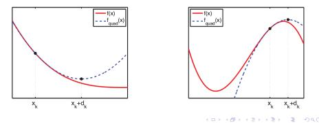
Algorithm 8.1: Newton's method for minimizing a strictly convex function
